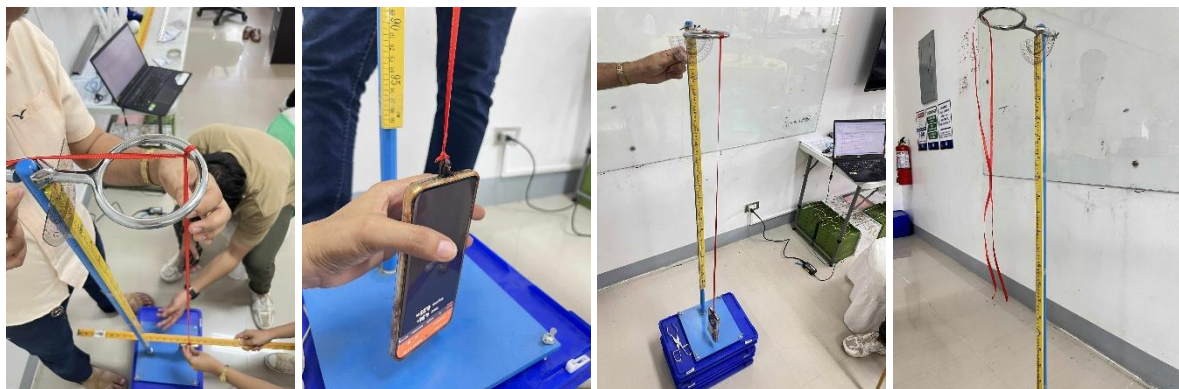
Figure 1. Experimental setup for determining the acceleration due to gravity using a smartphone-based pendulum system. The smartphone is attached to one end of a string and suspended from an iron stand, allowing it to oscillate freely. The Phyphox application is used to measure the time period of oscillation, with string lengths varied across six trials to compute gravitational acceleration.
